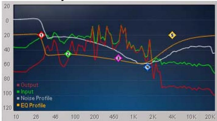
The Z-Noise Analyzer is the processor's main display. It shows four colored spectral envelopes:
