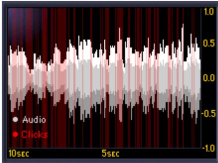
The X-Click Scope provides visual feedback for the last 10 seconds of processing history. Red denotes detected clicks; the intensity of the color corresponds to the degree of damage in the sample. The audio samples unaffected by X-Click are colored gray. Higher threshold values yield more red clicks displayed in the scope.
