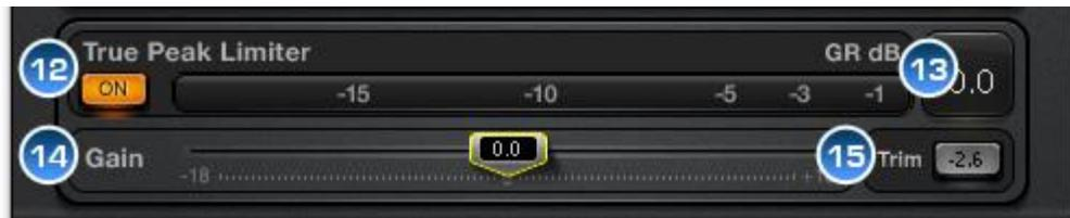
**12. True Peak Limiter** Activates the True Peak Limiter compliant with ITU 1770-3. The threshold is automatically defined by the “True Peak Max” value located in the “Settings Panel”. The True Peak Limiter is independent of the “Channels” setting and affects all channels. The limiter does not introduce make-up gain.
