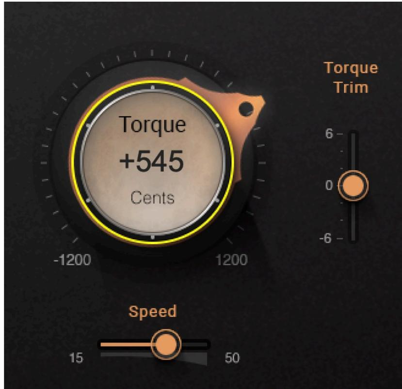
The **Torque Knob** controls the amount of formant shift. This action mostly affects the frequencies around the Focus setting. So if Torque is not correcting tone as expected, re-adjust the Focus setting. The amount of offset is displayed on the knob in cents. Range:  $\pm 1200$  cents
