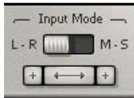
**LR/MS input button** - Changes input mode to accept either standard Left-Right inputs or Mid/Side (MS) inputs. See the chapter **About MS**.
