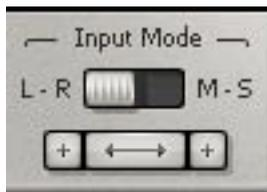
The standard S1 Shuffler or Imager can be used with input stereo signals from either standard left-right (LR) stereo or MS stereo. In both cases, the output is in standard left-right stereo mode. Click the button above the channel swap/polarity buttons to select which mode you need. In MS mode, what is normally the left input channel now accepts the M signal and what is normally the right input channel now accepts the S signal.
