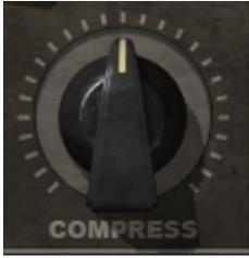
**COMPRESS** controls dynamics processing. Turning the knob clockwise results in more compression.
