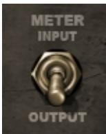
**METER SWITCH** toggles meter monitoring between input and output modes.
