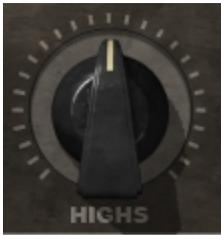
**HIGHS** controls high frequency equalization.
