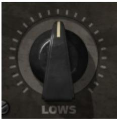
**LOWS** controls low frequency equalization.
