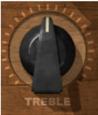
**TREBLE** controls the high frequency gain.
