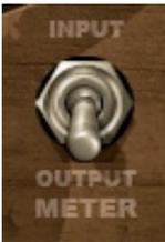
**METER Switch** toggles meter monitoring between input and output modes.
