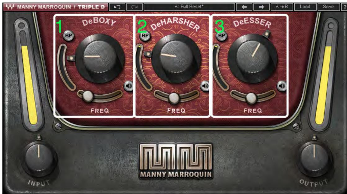
1. **DeBoxy Section** includes bypass, threshold, frequency, listening control and attenuation meter for DeBoxy processing.
