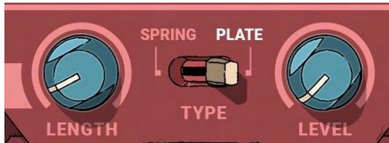
This unit features two types of IR reverb, with control over reverb tail length and overall level.
