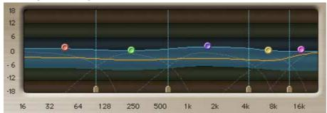
The MultiBand graph is like an EQ graph showing Amplitude in the Y-axis and Frequency in X-axis. In the Middle of the graph resides the DynamicLine<sup>TM</sup> that shows the per band gain adjustment as it happens within the Range, represented by the Bluish highlight. Beneath the graph there are the 4 Crossover frequency markers and on the graph there are 5 markers that allow you to set the gain of the band by dragging up and or down and the band's width by dragging sideways.
