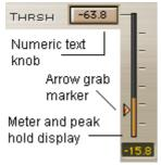
Each Band has its own meter showing the input energy in that band. Under the meter is a peak hold numeric indicator. When you want to set your nominal thresholds you can use the peak as reference and then continue to set them with the master threshold control.
