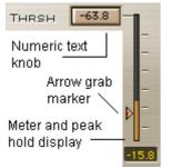
Defines the point of reference for that band's energy. Whenever the energy in a certain band exceeds the threshold gain adjustment will be applied. For your convenience, each band has an energy meter for visual adjustment of the Threshold
