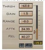
Each band of Waves LINMB has 5 adjustable dynamics settings. *Threshold*, *Gain*, *Range*, *Attack*, *Release*, *Solo* and *Bypass*. These function similarly in most dynamics processors but in this processor they affect the dynamics of one of the 5 bands. The *Range* may seem unfamiliar and basically it is in place of the well-known *Ratio*, but it defines both the intensity of gain adjustment and the limit of gain adjustment. Read more In the next chapter.
