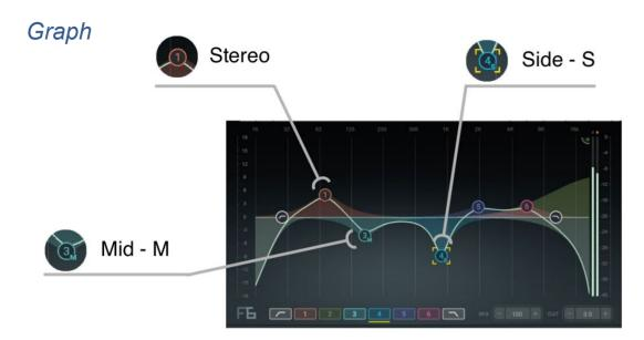
The Graph displays filters (Band Markers) and shows the effects of dynamic processing. Frequency is shown on the horizontal scale and amplitude on the vertical scale. The Total Curve Line provides a summary of the filters and dynamics for all bands.
