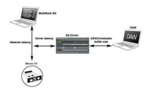
The above diagram illustrates the various latencies in the SoundGrid system. Network latency occurs between the I/O device and the processing engine; driver latency is added between the network and the host computer on which the driver is installed. ASIO or Core Audio buffering is usually added between the driver and the DAW software.
