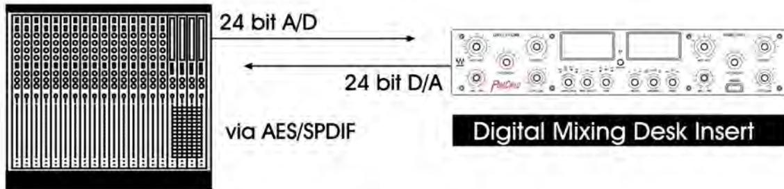
Connect a send point or an insert point from the mixing desk to the appropriate digital input of the PuigChild. Connect the PuigChild's digital output to the Send/Insert return point.
