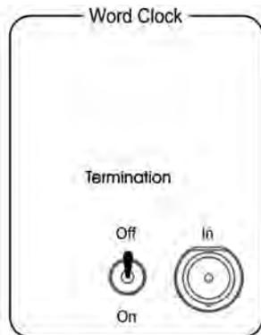
The PuigChild can be connected to an external word clock source (using a BNC connection) or you can use its internal clock. An external word clock is utilized for applications that require synchronization with other digital audio devices. The internal clock setting is selected on the front panel only when using the PuigChild's analog inputs.
