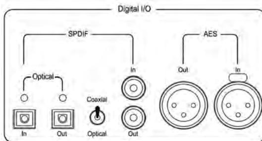
S/PDIF input/output uses either RCA or Optical connectors. The input format is selected using the Coaxial/Optical selector switch.
