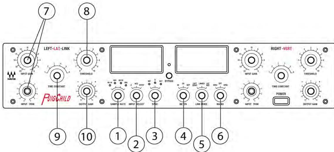
1. **Sample Rate** selects / displays the PuigChild sampling rate. PuigChild supports operating sample rates up to 96 kHz. You can only change the signal sample rate when the PuigChild's Sync mode is set to Internal. At the other settings the PuigChild locks to the digital stream or external Word Clock source. The PuigChild will automatically detect and display the sample rate for all other Sync modes.
