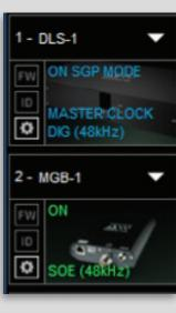
SoundGrid Studio uses Ethernet to stream audio between devices on a SoundGrid network. Synchronization clock is also carried over Ethernet. This method of providing clock is called Sync over Ethernet (SoE). SoundGrid I/O devices can be clocked by other means, but SoE is a more convenient way to provide clock information to devices on the SoundGrid network.
