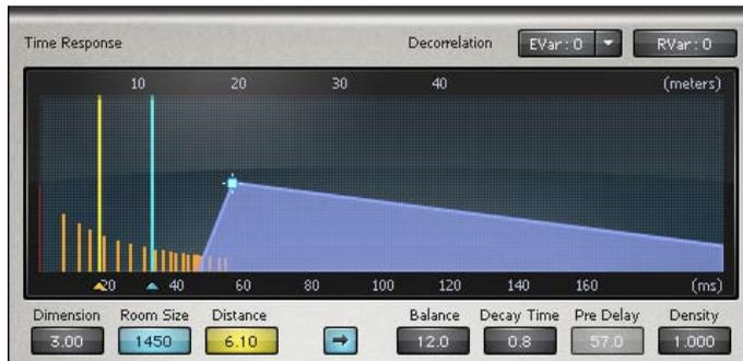
Room Size on the graph is shown at the top in meters (one axis) and the bottom in milliseconds; therefore, a size of 20 meters means a room 20x20x20=8000 cubic meters. The Room Size button, just below the Time window, shows the total cubic meter size. (Example: you want a small hall, 10 meters wide, 5 meter ceiling, and 20 meters deep = 1000 cubic meters).
