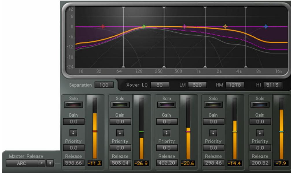
This section consists of the main display and controls for Separation, Xover, Solo, Gain, Priority, Release, and Master Release.
