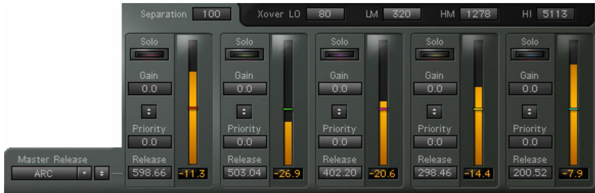
The Band Controls section features controls over the Crossover network which splits the input into Frequency Bands. Each Band has controls for Solo, Gain, Priority, Release, and a Meter displaying the input level.
