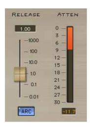
5 - Leave the ARC<sup>™</sup> (Auto-Release Control) engaged at all times unless you have a very specific type of limiter behavior, such as pumping or distortion effects. ARC calculates the release time every sample for optimum level with minimum artifacts. For nearly every possible source, ARC will outperform a fixed release time.
